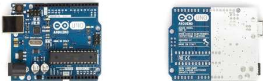
Figure 7: Arduino Uno Microprocessor Board (Front and Back)
