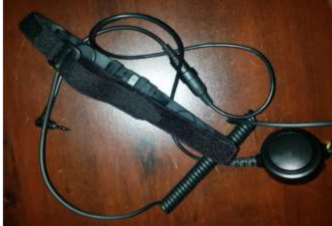
Figure 9: Throat Microphone with Two Sensors
